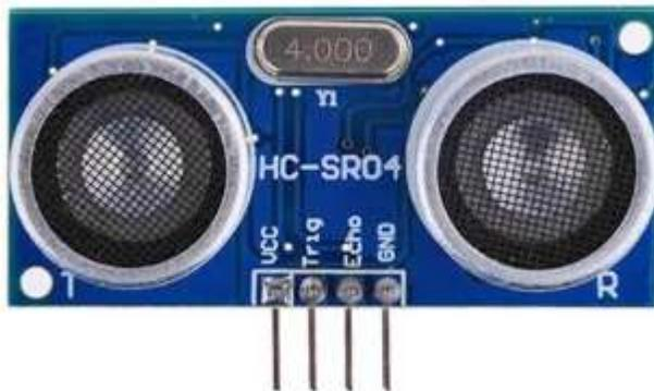
Figure 2.4: Sensor ultrassónico HC-SR04. (ElecFeaks, 2019)
